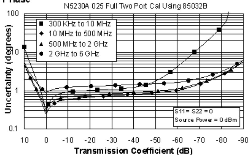
**NOTE:** The following graphs also apply to the "C" model of the analyzer.
